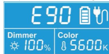
LCD screen displays dimmer, color temperature value, and remaining battery status. Pressing the knobs can switch to quick adjusting mode.
