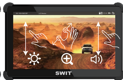
Left part up/down - Backlight adjust Right part up/down - Volume adjust Pinch with 2 fingers - Quick Zoom-in/out
